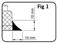
In order to maintain IPX9K protection, it is recommended that the integrity of the sealant is periodically checked and re-applied as necessary during the service life of the installation.
